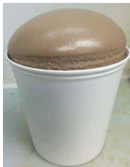
Fig. 6: Foam made of resin blend 14B96-2 that was aged for 110 days at 50 °C
