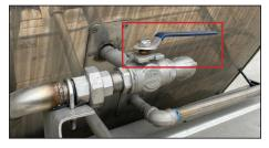
Blow Down Valve. Valve remains closed unless you are in the process of depressurizing (blowing down) the tanker.
